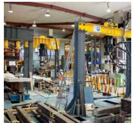
Strong Floor 8m x16m and associated Testing Rigs
